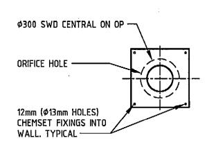
MATERIAL = GRADE 304 STAINLESS STEEL PLATE 6mm THICK
